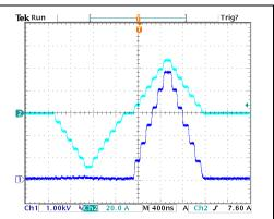
Bipolar pulse between two Channels, on a resistive load: (cyan) current, 20 A/div; 400 ns/div, (blue) voltage, 1 kV/div.
